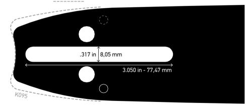
\*Note: In a few cases where two bars would have the same called length but different drive-link counts, the letter Z will be used in the motor-mount description to distinguish between them (K095 and Z095 for example).
